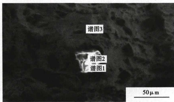
图3 断口上夹杂物点扫描图像 Fig.3 Spot scan image of inclusion at the fracture
